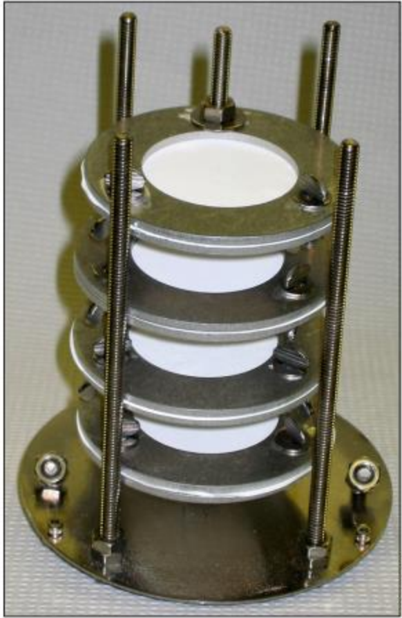
Figure 1 Polar Organic Chemical Integrative Sampler (POIS) housing with four sorbents. Source: https://www.cerc.usgs.gov/pubs/center/pdffdocs/pocis.pdf , 3/16/2022
